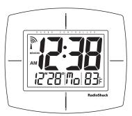
For about 2 minutes after you install the batteries, the clock scans for the radio signal while  $\mathbb{P}$  flashes.
